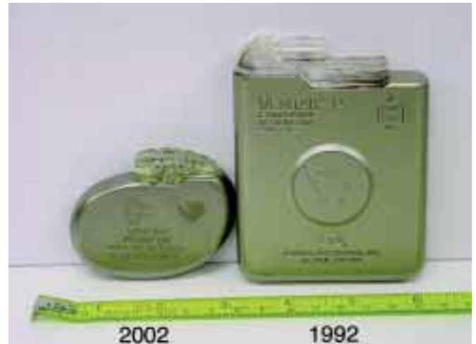
Changes in ICDs over 10 years (1992–2002). Apart from reduction in size, the implant technique and required hardware have also improved—from the sternotomy approach with four leads and abdominal implantation to the present two-lead transvenous endocardial approach that is no more invasive than a pacemaker requires
